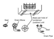
Fit the seal into the drain elbow, then insert the drain elbow into the base pan hole of the condensor (outdoor) unit, rotate 90° to securely assemble. Connect the drain elbow with an extension drain hose (locally purchased), in case the water drains off the condensor (outdoor) unit during the heating mode. (heating models only).
